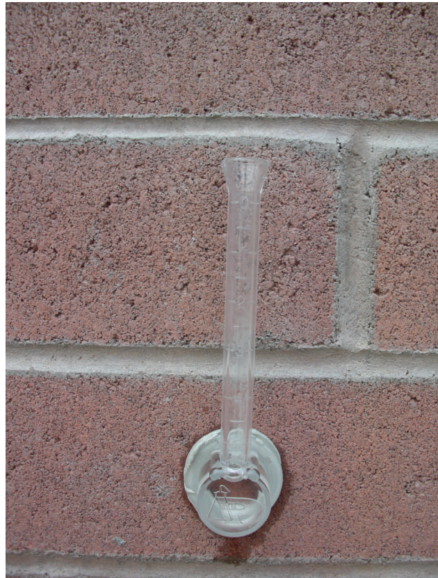
Rilem tube used to measure absorption of a vertical surface
