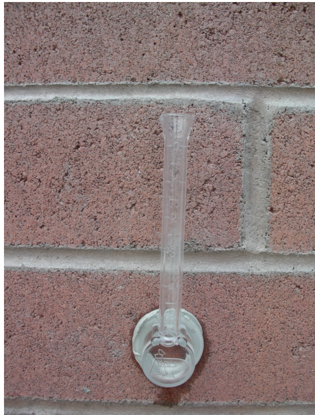
Rilem tube used to measure absorption of a vertical surface
